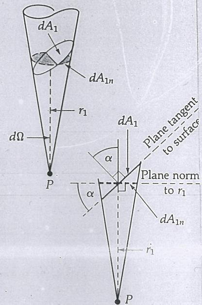
(c) The area  $dA_{1n}$  is the projection of the area  $dA_1$  on the plane perpendicular to  $r_1$ . It equals  $dA_{1n} = dA_1 \cos \alpha$ .
