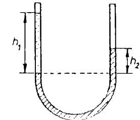
$$\rho_1 g h_1 = \rho_2 g h_2 \quad \text{ali} \quad \rho_1 = \rho_2 h_2 / h_1 = 1,0 \text{ g/cm}^3$$
