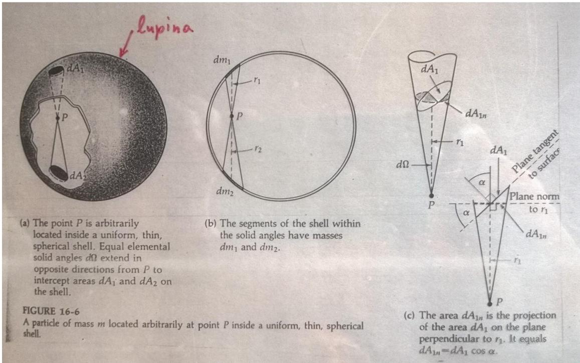
$$dm_1 = \sigma dA_1 = \frac{\sigma d\Omega r_1^2}{\cos \alpha} \quad \text{and} \quad dm_2 = \sigma dA_2 = \frac{\sigma d\Omega r_2^2}{\cos \alpha}$$
