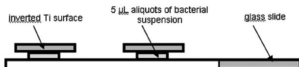
**Fig. 1 – The incubation procedure for bacterial adhesion tests. Test surfaces were inverted onto droplets of a bacterial suspension in artificial saliva on microscope slides contained in a Petri dish as shown for 1 h.**
