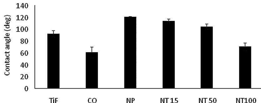
**Fig. 4 – Mean water contact angles and associated standard deviations obtained on the nanopore (NP), compact oxide (CO) and Ti foil (TiF) and nanotube (NT) surfaces ( $n=15$ ). All results were significantly different from each other ( $p<0.05$ ).**
