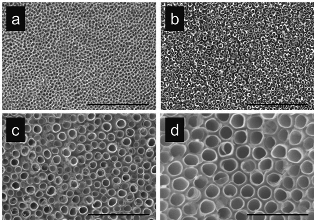
Fig. 2 – SEM images of the upper surface of  $\text{TiO}_2$  nanostructures of different diameters: (a) 15 nm NP, (b) 15 nm NT, (c) 50 nm NT, (d) 100 nm NT (NP: nanopores, NT: nanotubes), Scale bar: 500 nm.
