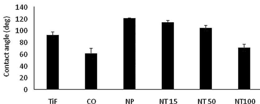
Fig. 4 – Mean water contact angles and associated standard deviations obtained on the nanopore (NP), compact oxide (CO) and Ti foil (TiF) and nanotube (NT) surfaces ( $n = 15$ ). All results were significantly different from each other ( $p < 0.05$ ).
