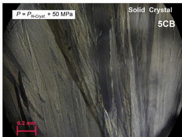
Fig. A3.5. Polarization microscopy insight into pentylcyanobiphenyl (5CB) on compressing: the solid crystal phase.
