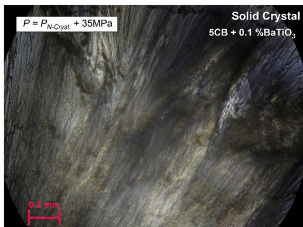
**Fig. A3.10.** Polarization microscopy insight into pentylcyanobiphenyl (5CB) and 0.1% of BaTiO<sub>3</sub> nanoparticles ( $2r = 50nm$ ) on compressing: the solid crystal phase.
