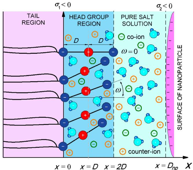
**Fig. 1.** Schematic presentation of the model to study the interaction between negatively charged POPS lipid and negatively charged NP suspended in salt solution. Negative charges at  $x=0$  are described as negative surface charge density  $\sigma_1$ .  $D$  is the distance between opposite charges within the head region,  $\sigma_2$  is the surface charge density of charged NP, while  $\omega$  describes the orientation angle of the single head group.
