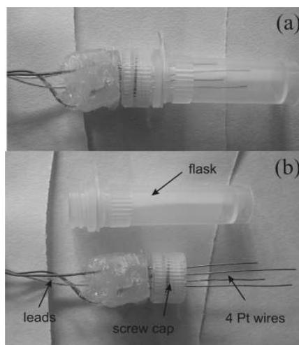
**Figure 3.** Electroformation cell with 4 Pt electrodes.
