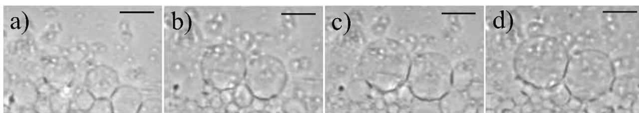
Fig. 5. Micrographs depict solution containing magnetoliposomes with positively charged magnetic nanoparticles prepared at 5 V and 3 Hz in time (a) after 10 min of electroformation, (b) 20 min, (c) 30 min and (d) 40 min. Bar is 10  $\mu$ m, optical magnification is 1000 times.
