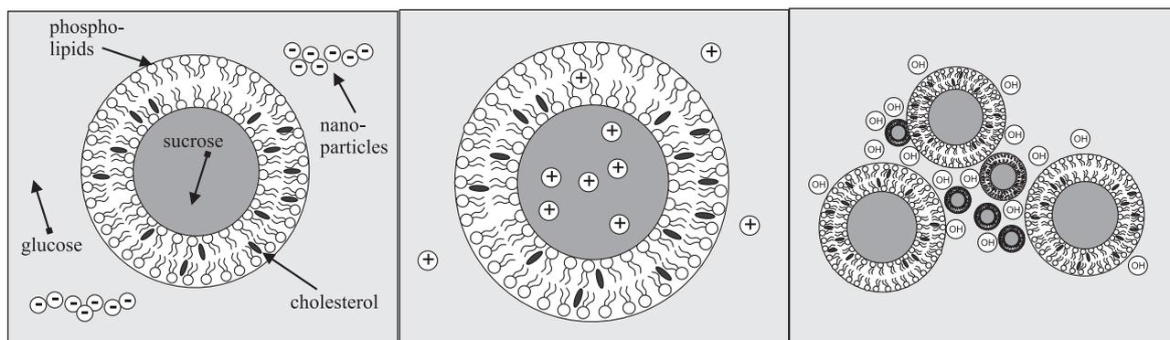
**Fig. 6.** Models of interaction of various nanoparticles with phospholipid vesicles are schematically presented. Left cartoon shows liposomes with negatively charged magnetic nanoparticles; middle cartoon shows liposomes with positively charged magnetic nanoparticles; right cartoon shows liposomes with magnetic nanoparticles functionalised with  $-OH$  groups on the surface.
