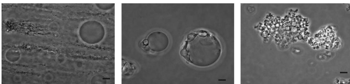
**Fig. 7.** Left micrograph presents solution containing liposomes with negatively charged magnetic nanoparticles. Middle micrograph presents solution containing liposomes with positively charged magnetic nanoparticles. Right micrograph presents solution containing liposomes with  $-OH$  groups on the surface of nanoparticles. Bar is 10  $\mu m$ , optical magnification is 1000 times.
