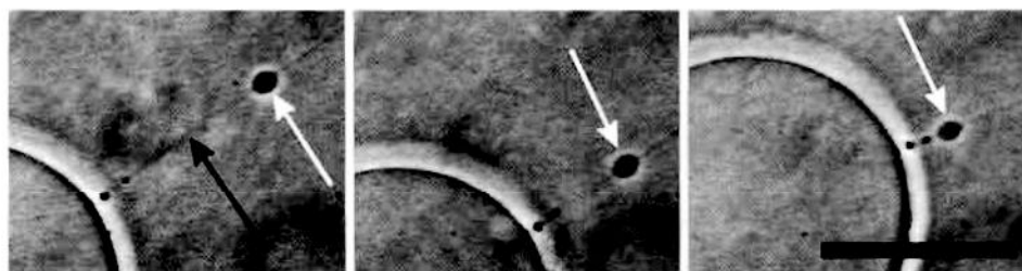
Fig. 15. Movement of a small phospholipid prolate carrier vesicle (white arrow) along a thin phospholipid tube (black arrow) attached to a giant phospholipid vesicle (adapted from [52]). Scale bar = 10 \mu\text{m} .
